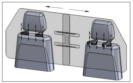
**STEP 6:** Once Car Shield is secured to each Headrest with the Hook and Loop Fasteners, go back and tighten hardware using Phillips head screwdriver and supplied wrench.
